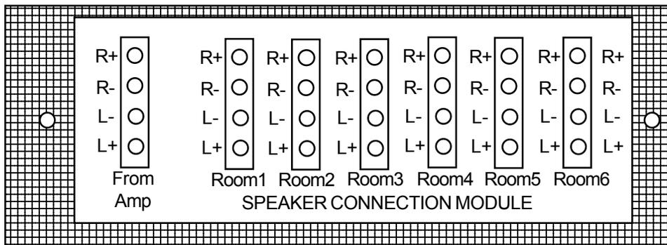
The **WT6** can be used to connect multiple speakers to an amplifier, multiple infrared receivers to a connection block or any other low voltage multiple application. All of the WT6 R+ terminals are connected together, as are the R-, L- and L+ terminals.
